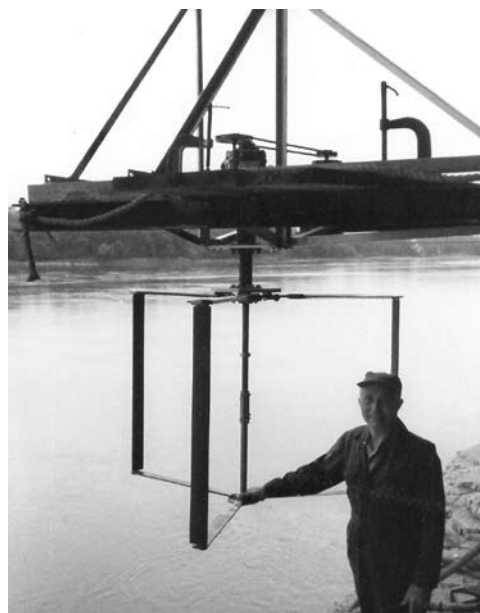
Mod-1 test in the Missouri River of an Aquagiro mounted on a boat-cart ramp
